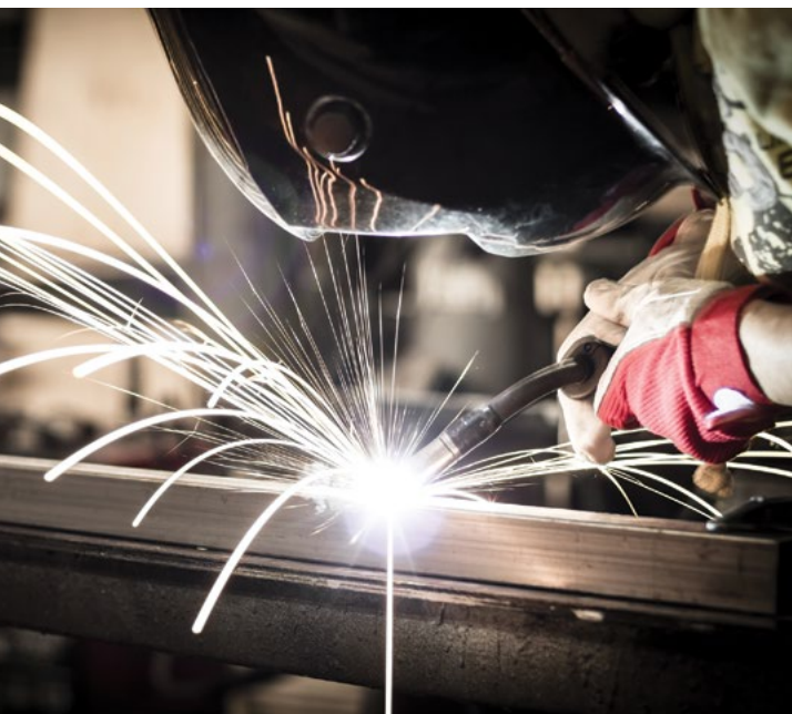
Exposure to welding fumes and gases may be acute or prolonged. Acute exposure can cause eye, nose and throat irritation, dizziness and nausea. (photo courtesy Adobe Stock)
